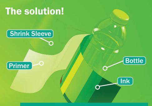
Our solution is simple. We make the ink separate itself from the shrink sleeve. But we want to make sure this only happens in the recycling process. That way the ink and the sleeve can go separate ways. The sleeve material goes with the bottle material and the ink is removed with the caustic wash.
