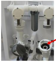
4. The chemical lines stay connected and you have access to the backflow preventer assembly.
