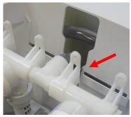
2. Lift the engine up off the joggle bracket. The water line remains connected.
