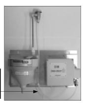
Use a 3/8" ID garden or utility water hose to connect the incoming water supply to the inlet side of the solenoid. Slip the blunt end of hose over the brass barb and secure it with a hose clamp. *Note:* Maximum water pressure is 40 PSI;
