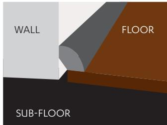
**QUARTER ROUND** is most commonly applied to cover the expansion gap between the flooring and the wall.
