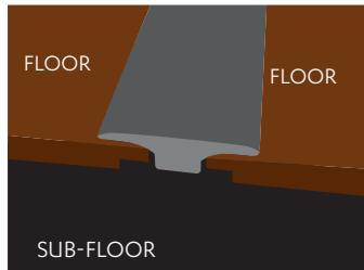
**T-MOLD** is used when joining two floors of equal height, such as in a doorway, between two rooms or in a large area where the maximum length/width is exceeded.
