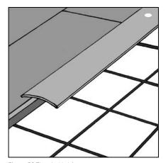
Figure 58 Threshold strip
