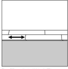
Figure 5 Stagger the short joints min 150mm
