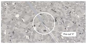
Figure 3 Weld joins
