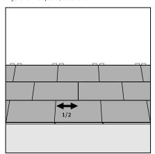
Figure 16 Stagger the short joints
