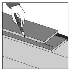
Figure 6 Last row, cutting the plank/tiles
