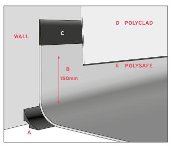
Figure 2 Overlap installation method
