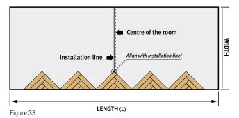
▶ Lay out the triangles with their long side towards the starting wall. Align the tip of centre triangle with the installation line. Position spacers between the wall and the triangle bases.
