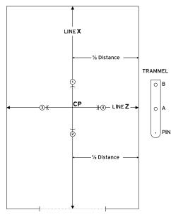
Figure 6 Marking out straight tiling
