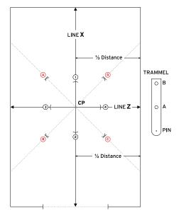
Figure 7 Marking out diagonal tiling
