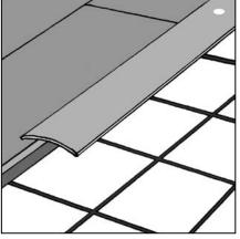
Figure 23 Threshold strip
