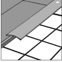
Figure 10 Threshold strip
