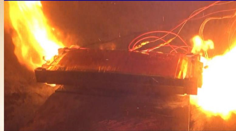
EV pouch cells undergo particle emissions testing
