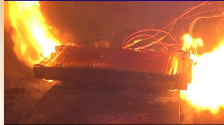
EV pouch cells undergo particle emissions testing
