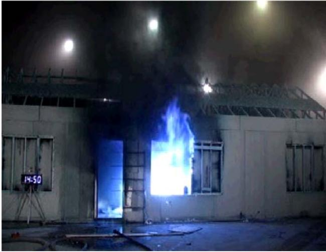
Figure 509. Conditions after ventilation of window (14:50)
