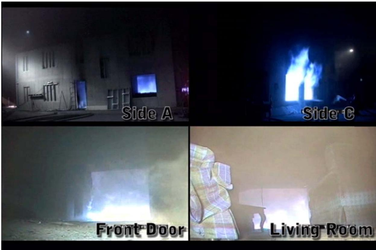
Figure 528. Two-story house before fog stream application (Experiment 15)
