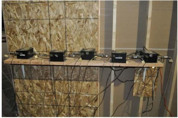
**Figure 162. Pressure Transducers**
