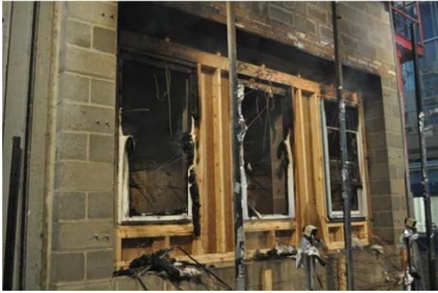
**Figure 69. Exp. 4 Post experiment, Unexposed side**
