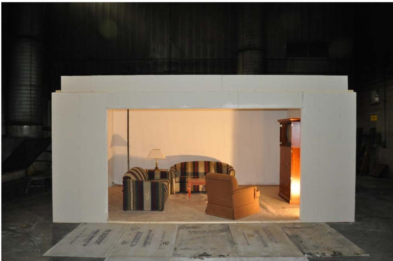
Figure 126. Heat Release Rate Experimental Set-up
