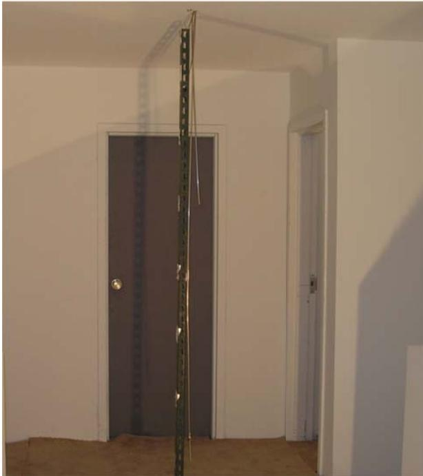
**Figure 163. Gas Sampling Tubes**
