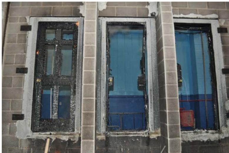
**Figure 75. Post experiment photo of the doors**
