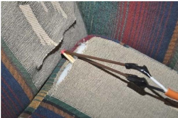
**Figure 168. Remote Ignition Device**
