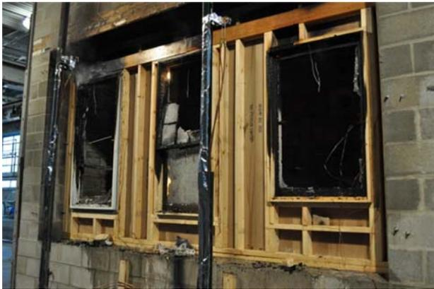
Figure 67. Exp. 3 Post experiment, Unexposed side
