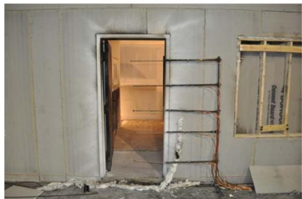
**Figure 160. Doorway Velocity Probes**
