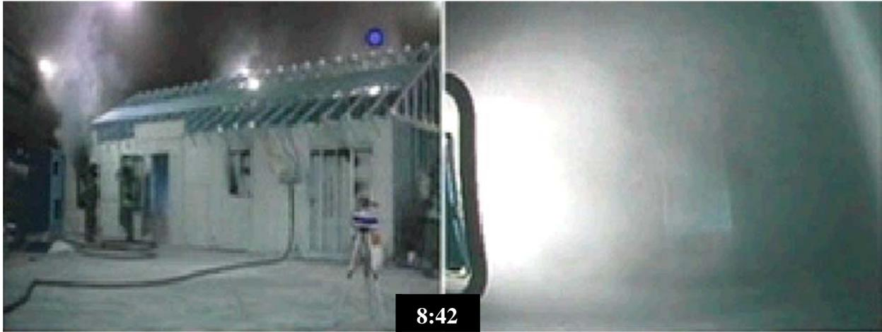
Figure 495. Experiment 14 view of rear of house and Bedroom 3 at 8:42
