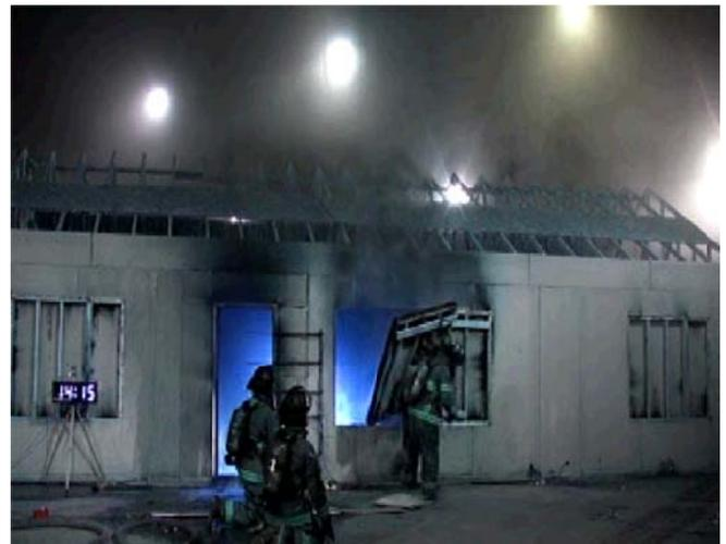
Figure 508. Conditions at time of window opening (14:15)
