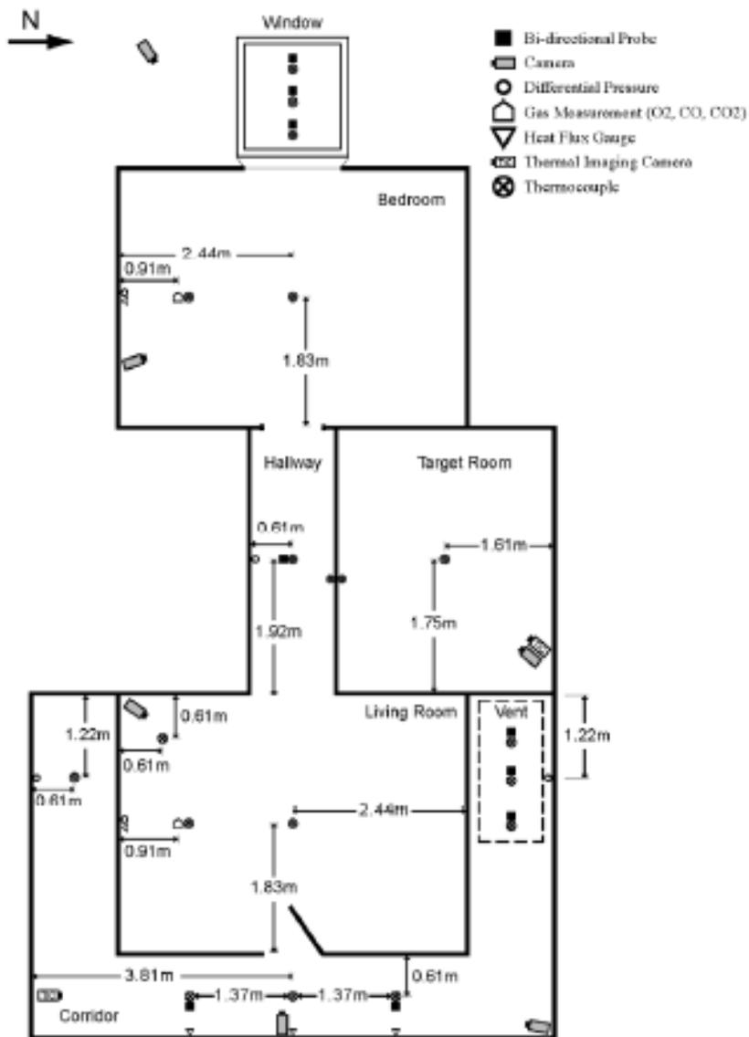
Figure 2.1: Residential apartment arrangement and instrument locations.
