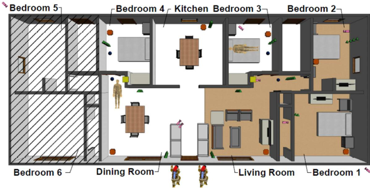
Figure 2.15: Floor plan with instrument locations for the IFSI, UL FSRI, NIOSH thermal response study. The room labels correspond with the measurement locations cited in Table 2.10. Fires were located in Bedrooms 1 and 2, or Bedrooms 5 and 6. [41].
