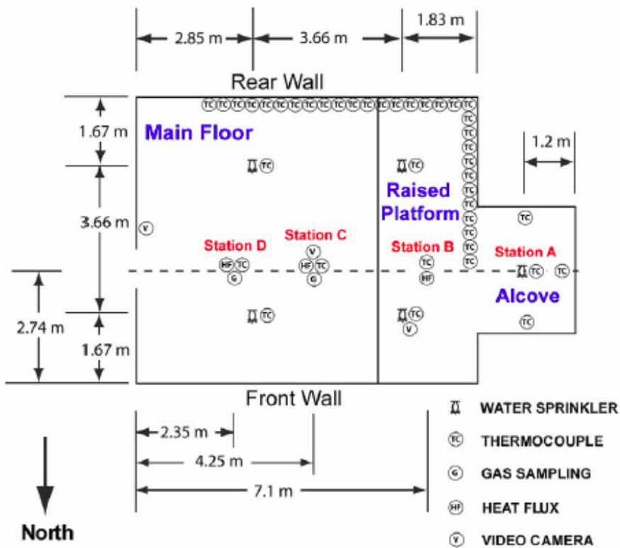
Figure 2.9: Public assembly occupancy plan view and instrumentation locations.
