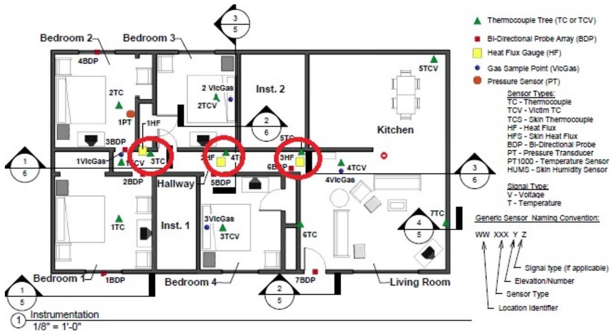
Figure 2.14: Floor plan with instrument locations for the UL FSRI fire attack study. The red circles indicate the measurement locations cited in Table 2.7. Moving from the front door toward the bedrooms, the locations are start, middle, and end of hallway, respectively. Fires were located in Bedroom 1 or Bedroom 1 and 2. [39].
