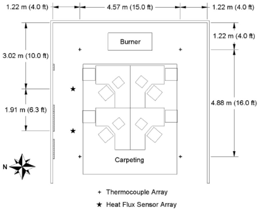
Figure 2.7: Open office plan arrangement and instrument locations.
