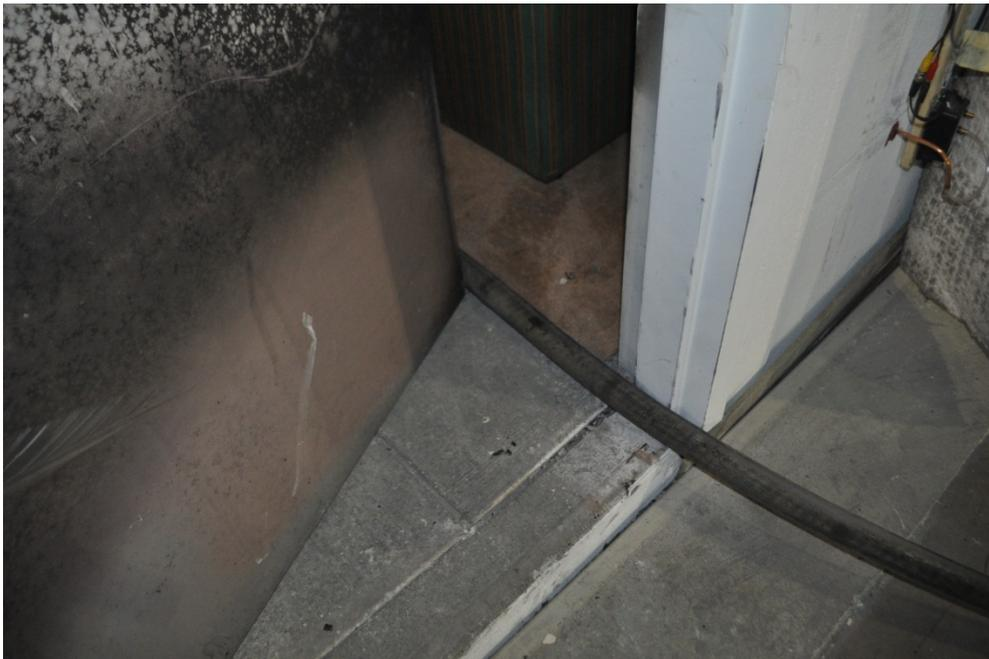
**Figure 4.2: Door Control with a 1 3/4 inch Hoseline**
