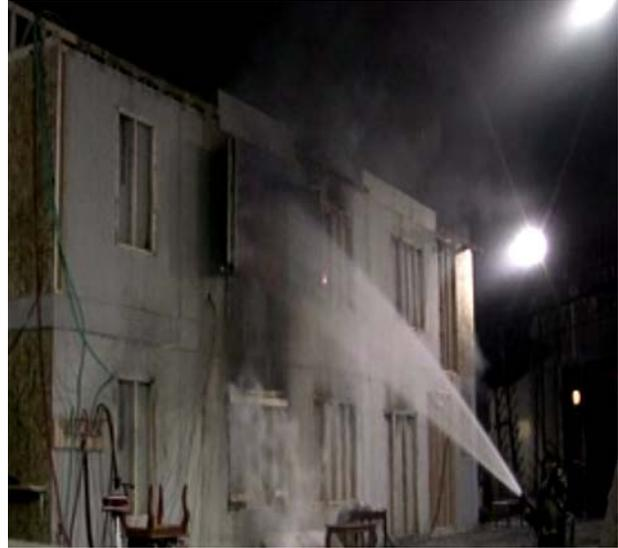
**Figure 4.36: Fog Stream Sealing Flow Path**
