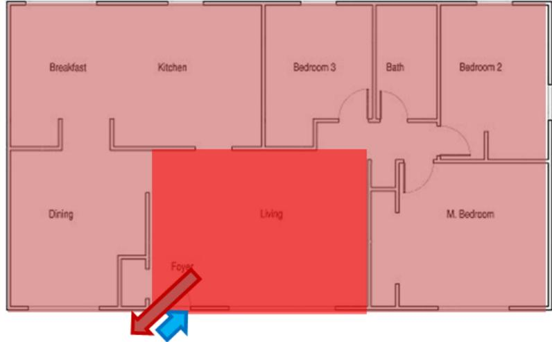
Fully Developed Stage: Ventilation-limited Fire. Flames extend out of doorway, inside house is too fuel rich to burn but continues to increase in temperature
