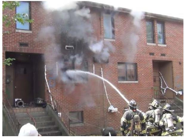
**Figure 4.38: Smooth bore being Whipped in a circular pattern blocking flow path out of Fire room**
