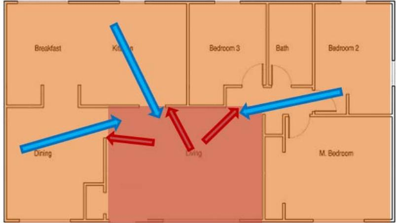
Initial decay stage: Ventilation-limited Fire. Room on fire, oxygen is running out and temperatures are dropping
