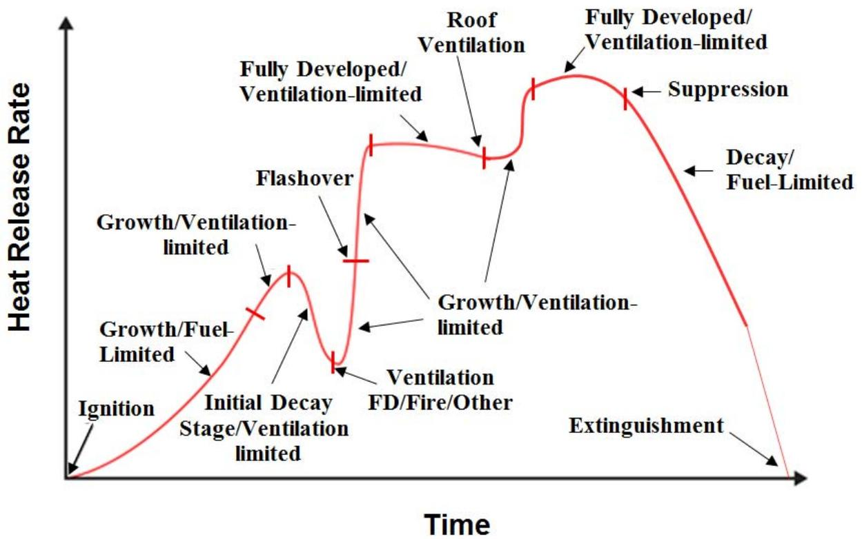
Figure 4.12: Fire growth curve for this fire example
