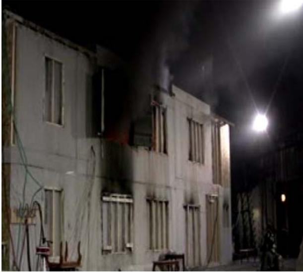
**Figure 4.35: Flow path before Water Application**
