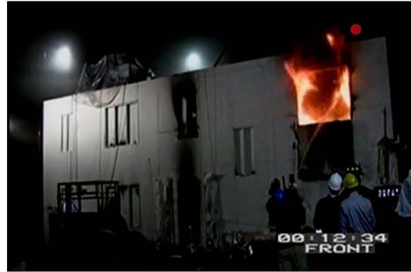
Figure 4.28: Water being applied from outside the house
