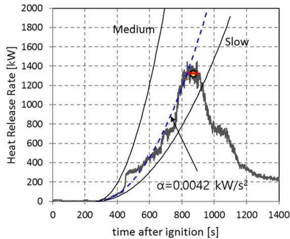
Figure 12. The measured heat release rate of a full-scale kitchen fire using a 3 kW ignition source in the presence of cabinets and the absence of a heated cooking oil fire [22].
