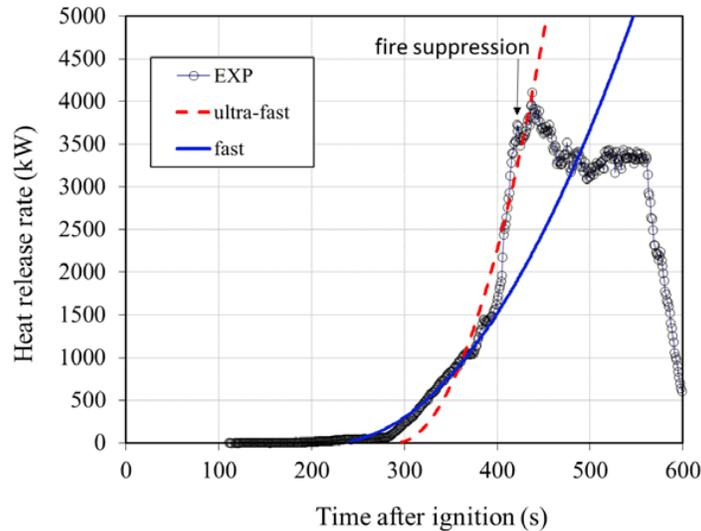
Figure 11. Comparison of the measured heat release rate and the  $t^2$  fire growth model during the full-scale kitchen compartment fire (Test KSG20) burning 1.6 L of corn oil in Pan B. A value of  $\alpha = 0.187 \text{ kW/s}^2$  indicates “ultra-fast”  $t^2$  fire growth.
