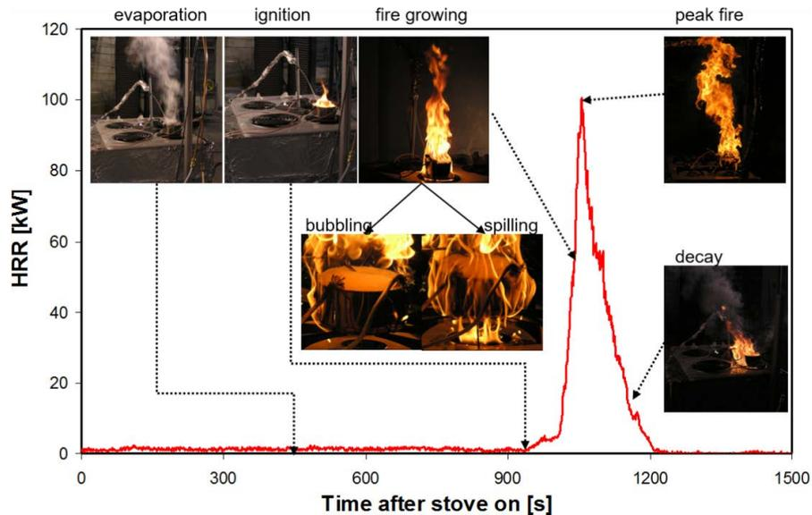
Figure 4. The measured heat release rate as a function of time for corn oil in Pan C. Photographs of key aspects of fire behavior are also shown.
