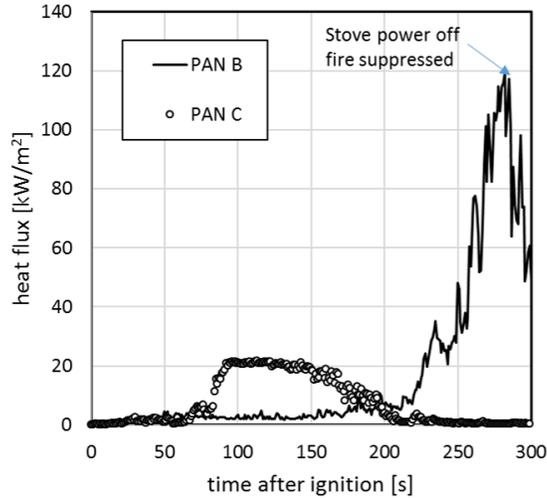
Figure 7. The evolving heat flux measured at the heat flux location 2 after ignition for corn oil.
