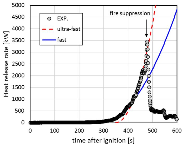
Figure 10. Comparison of the measured heat release rate and the  $t^2$  fire growth model during the full-scale kitchen compartment fire (Test KSG15) burning 4.5 L of corn oil in Pan A. A value of  $\alpha = 0.187 \text{ kW/s}^2$  indicates “ultra-fast”  $t^2$  fire growth.
