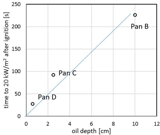
Figure 8. Comparisons of the time required to reach a heat flux of  $20 \text{ kW/m}^2$  on heat flux gauge HF#2 (see Figure 1) as a function of oil depth on the electric cooktop.
