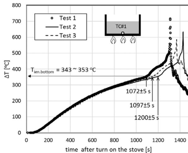
Figure 5. The evolving temperature measured at the bottom of Pan C with corn oil for Tests 1 -3.
