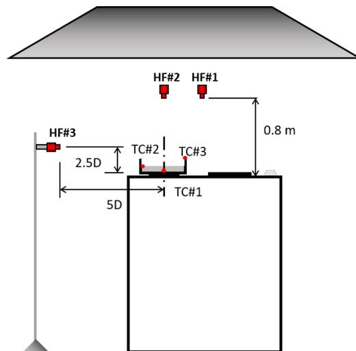
Figure 1. Schematic diagram of the apparatus used for stovetop fire characterization.
