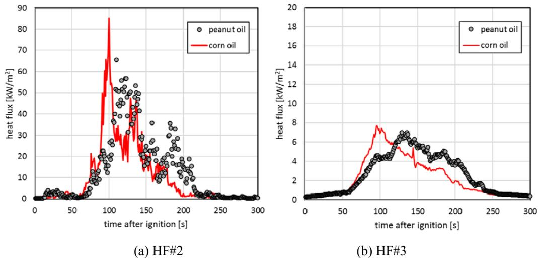
Figure 6. The measured heat flux at locations #2 and #3 (see Figure 1) for peanut and corn oil in Pan C.
