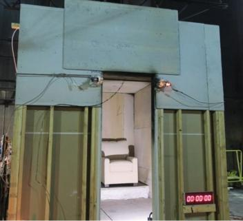
**Fire performance tests** were conducted in an ISO 9705 Test Room setup. Both open flame tests and cigarette smoldering tests (according to TB 117–2013) were conducted. Heat and smoke release rates, total weight loss, gas emissions, smoke yield and chemical and dust emissions in the fire effluents were measured.
