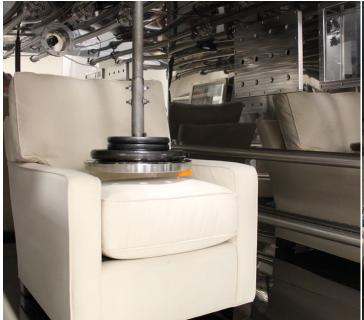
Chemical exposure testing was conducted in anFinenvironmental exposure chamber. Both VOC and aldehydeTeair emissions and flame retardants were measured.snDuring chemical sampling, the chairs were agitated using acospecially designed robot to simulate activity from daily use.los
