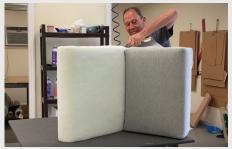
**3.** The cover fabric and fire barrier are installed at once, entirely encapsulating the foam cushion.
