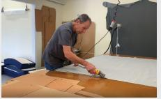
**1.** The fabric pattern (flatwork) for the chair seat cushion is cut out of the cover fabric laminated with the fire barrier.
