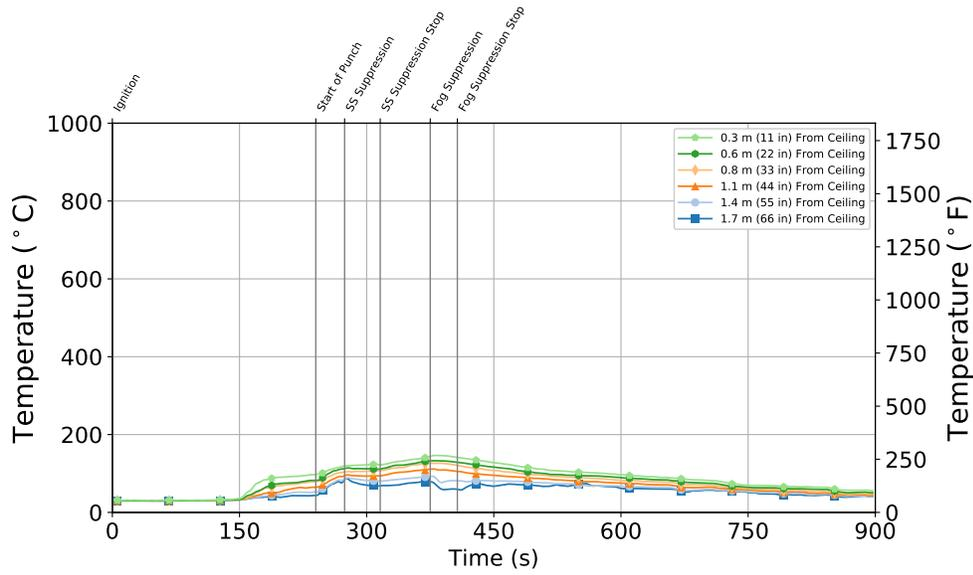
Figure B.111: Experiment 7 - Front Door Thermocouple Temperature at First Floor
