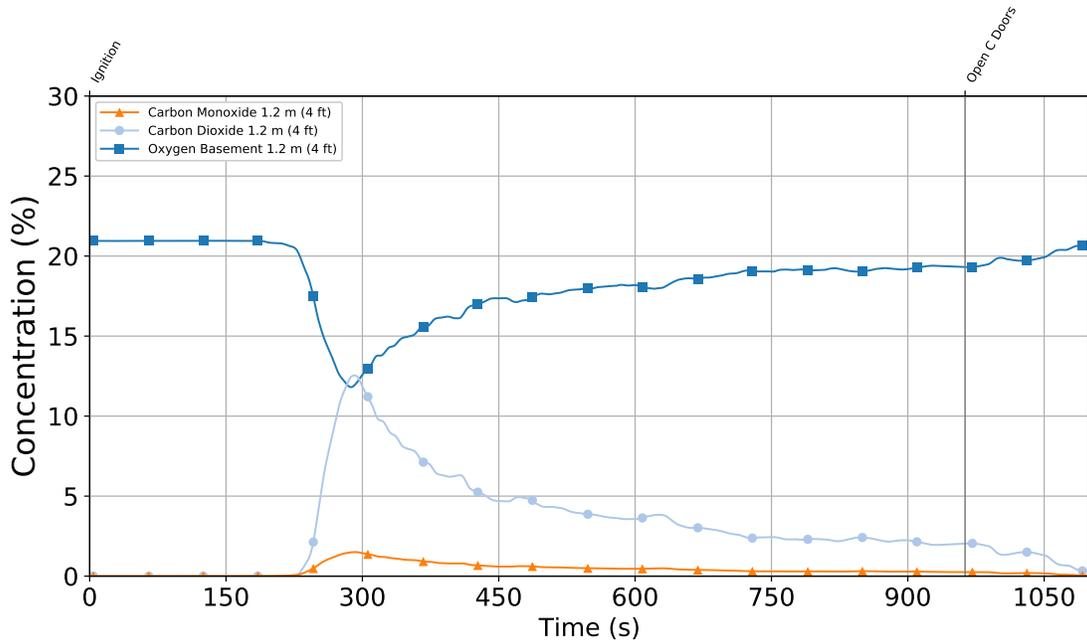
Figure 6.9: Experiment 5 - Gas concentration in the basement 1.2 m (4 ft) above the floor.
