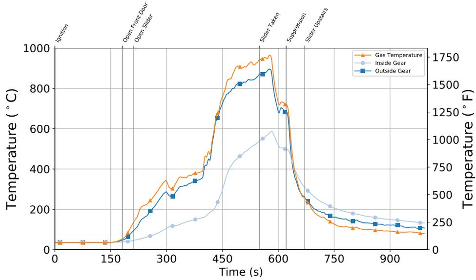
Figure B.130: Experiment 8 - Thermocouple Temperature on Inside and Outside of PPE Sample
