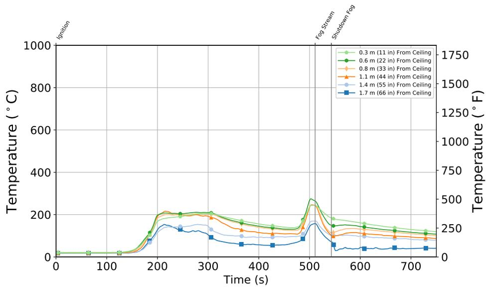
Figure B.187: Experiment 12 - Stair Thermocouple Temperature at First Floor
