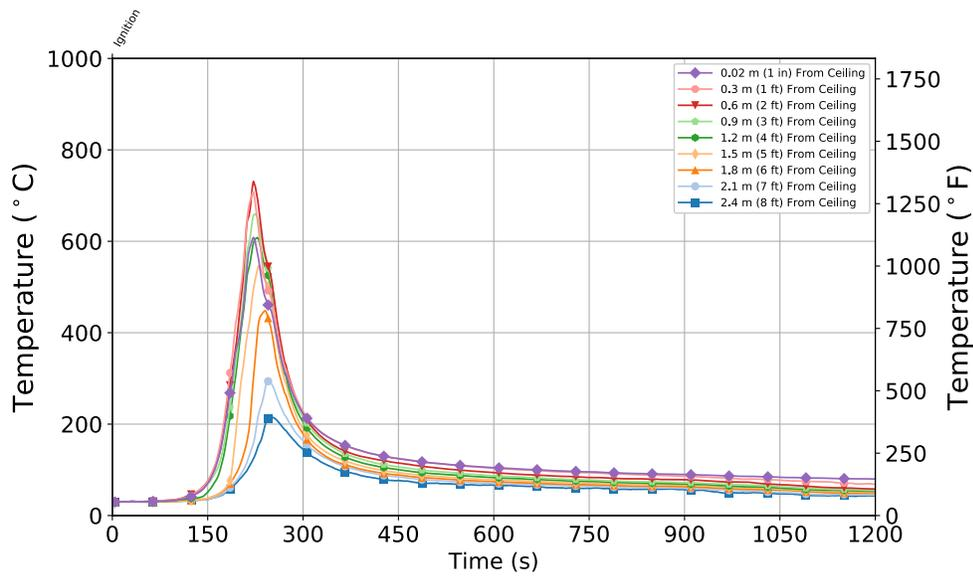
Figure B.36: Experiment 3 - Thermocouple temperature time histories from the Quadrant D thermocouple array in the basement.
