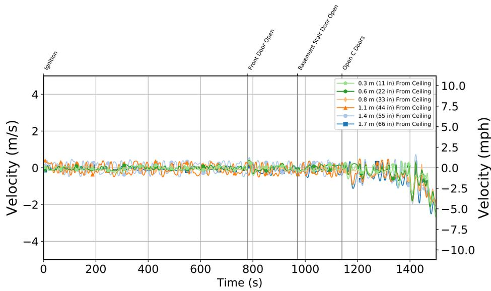
Figure B.13: Experiment 1 - Front Door Velocity at First Floor
