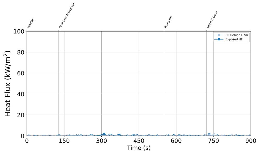
Figure B.160: Experiment 10 - Comparison of Heat Flux between Exposed Sensor and Protected Sensor
