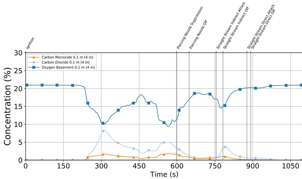
Figure B.139: Experiment 9 - Gas concentration time histories from the 1.2 m (4 ft) (top) and 0.1 m (4 in.) (bottom) elevations in the basement.
