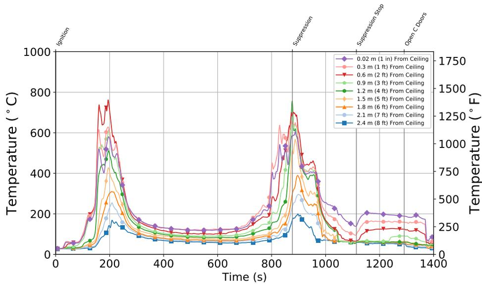
Figure B.165: Experiment 11 - Thermocouple temperature time histories from the Quadrant B thermocouple array in the basement.
