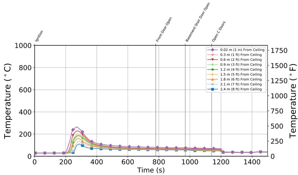
Figure B.1: Experiment 1 - Thermocouple temperature time histories from the Quadrant A thermocouple array in the basement.
