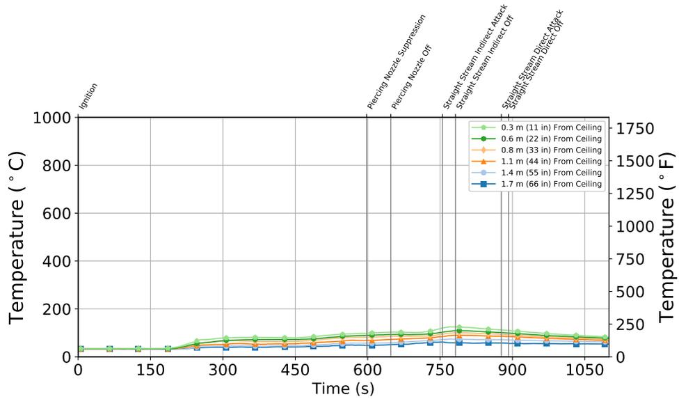
Figure B.146: Experiment 9 - Front Door Thermocouple Temperature at First Floor
