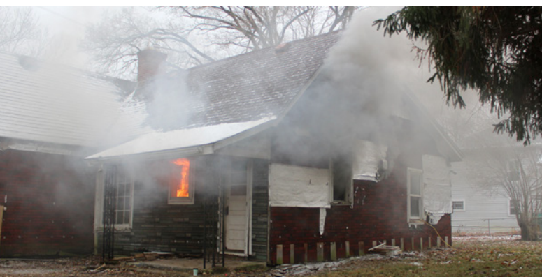
Figure 1. A photograph of an experiment from a kitchen fire in a single-story residential structure that has two open kitchen windows (single-family Experiment 16), and a representation of flows (intake and exhaust). After the rooms of the house open to the fire room have filled with smoke, the kitchen windows served as the only intake and exhaust vents of the flow path (shaded in gray).
