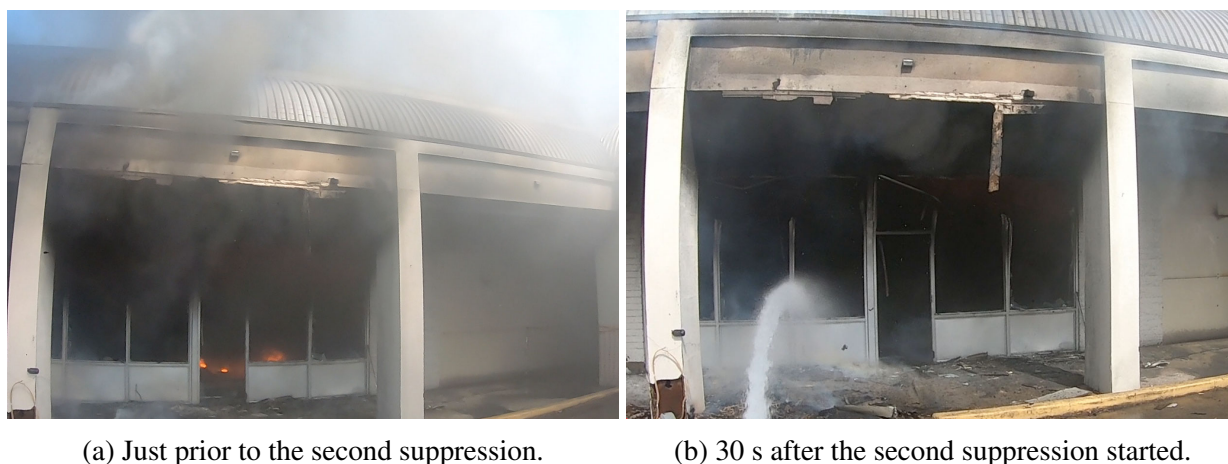
Figure 3.41: Conditions from the viewpoint of the nozzle firefighter at 12 min 21 s, just prior to initiating the second exterior water application, along with 30 s later (Experiment 4).
