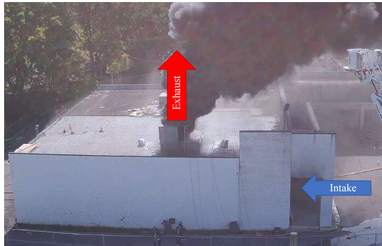
Figure 4.26: Flow path after initial vertical ventilation during Experiment 6 with the front door as a unidirectional intake and the open two roof vents as a unidirectional exhaust.
