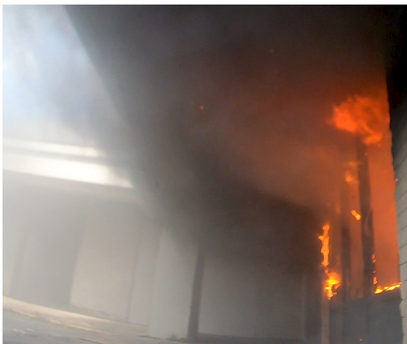
Figure 4.4: An image of flames venting out of the open front windows and door 18 min after ignition (Experiment 2).
