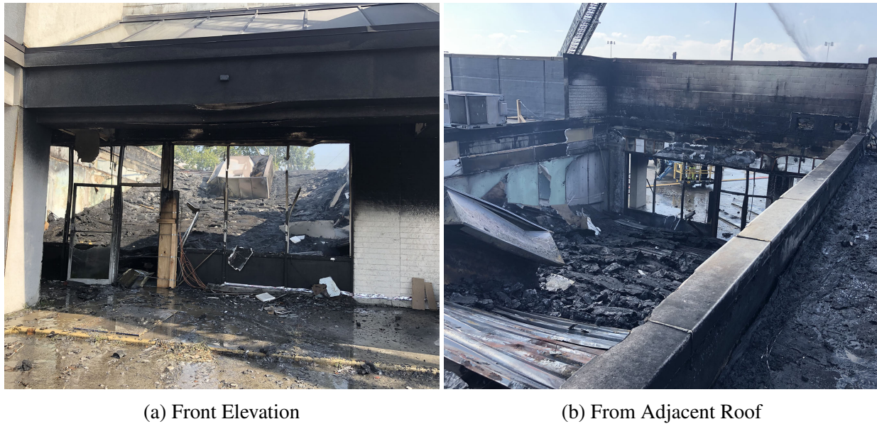
Figure 3.21: Images of the lean-to front roof collapse that occurred during Experiment 2.
