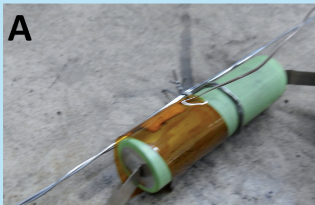
Figure 4. Comparison of an overcharge test on authentic (A) and low-quality (B) cell show the difference in the safety of these cells. Electrolyte leak, high heat, and fire is observed in case of low-quality cell.
