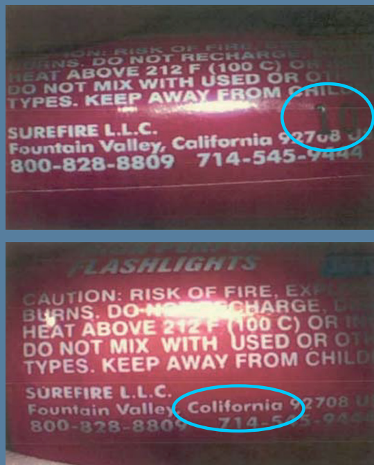
Figure 1. Comparison of a cell from an authentic US brand to a counterfeit. The counterfeit product shows a misspelling of California ("Colifornia") and a missing date stamp. 1
