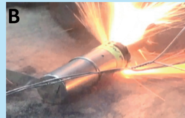
Figure 4. Comparison of an overcharge test on authentic (A) and low-quality (B) cell show the difference in the safety of these cells. Electrolyte leak, high heat, and fire is observed in case of low-quality cell.
