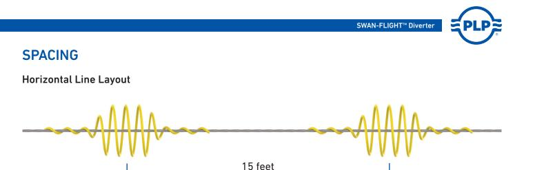
For optimal results, spacing distances are generally recommended at 15-foot intervals, depending upon local conditions. Since wind resistance is very limited, sufficient SWAN-FLIGHT Diverters can be used to ensure adequate visibility without creating stresses on the line. When marking adjacent spans, overall visibility is improved by staggering the placement between the spans.
