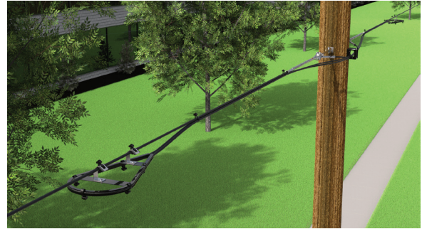
In-Span Storage Installed on ADSS Cable
