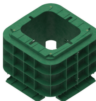
Catalog Number: COYGLC-B-000 COYOTE GLC Small Base 17" W x 17" L x 13" H (430 x 430 x 330 mm) For Fiber Optic Cables with Diameters up to 0.60" (15.2 mm)
