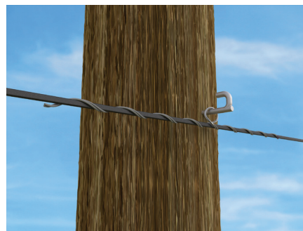
Standard Tangent Support with Flat Drop Cable
