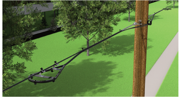
In-Span Storage Installed on ADSS Cable
