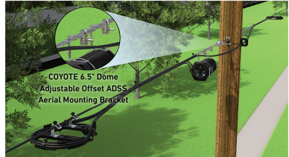
In-Span Storage Installed on ADSS Cable
