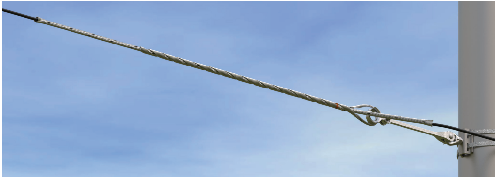
FIBERLIGN Medium Tension Dielectric Dead-End Installed on Steel Pole with Thimble Clevis, Extension Link, and Banding Bracket
