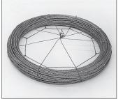
**3.** Twist at least 2" of the legs together until the wire cage is tight.
