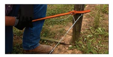
Building, extending, or repairing a fence is easy with the heavy-duty Ranchmate® Post Wire Stretcher for high-tensile steel wire.
