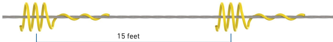
For optimal results, spacing distances are generally recommended at 15-foot intervals, depending upon local conditions. Since wind resistance is very limited, a sufficient number of BIRD-FLIGHT Diversers can be used to ensure adequate visibility without creating stresses on the line. When marking adjacent spans, overall visibility is improved by staggering the placement between spans.
