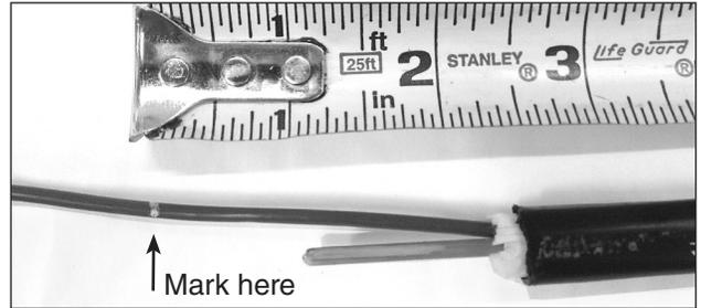
**Step #7** Align the strength member with the edge of the bracket (about 3/4") and trim.
