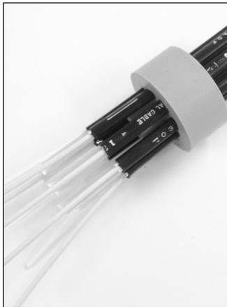
**Step #19** While cap is loose, insert all strength members under cap.
