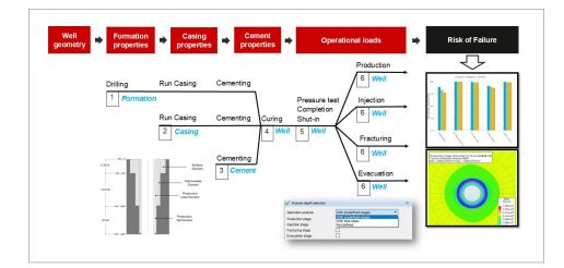
Life-of-the-well integrity workflow illustrates how WellLife® software, a well integrity digital twin, enables the construction and evaluation of the well's potential for failure (i.e., remaining capacity) during its productive life.
