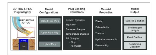
Abandonment integrity workflow indicates how WellLife® software helps analyze a plug's potential for mechanical or poro-mechanical failure as a wellbore is decommissioned.
