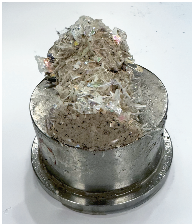
Figure 3. Physical lab tests confirm the LCM package and concentration's ability to seal the expected geometry.
