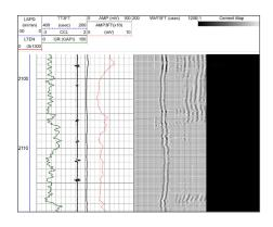
Excellent CBL result with readings of <10 mV across the shoe and proved bonding by a successful formation integrity test (FIT).
