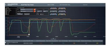
Real-time viewer provides remote access to real-time data and calculated variables. Real-time pressure match assessment between design and execution allows the viewer to instantly evaluate TOC compliance with requirements and enables real-time insights into the cement operation, which facilitates prompt decision-making and the capability to addresses potential issues before they escalate.
