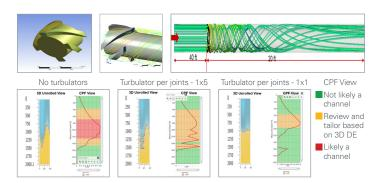
Predictive diagnostics with turbulator and Protech™ centralizers. This characterization demonstrates the impact of turbulator-like geometries on fluid intermixing profiles, which, in some cases, can eliminate the need for additional pipe movement aids.
