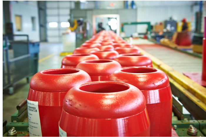
Float equipment production line at Halliburton Houston manufacturing plant.
