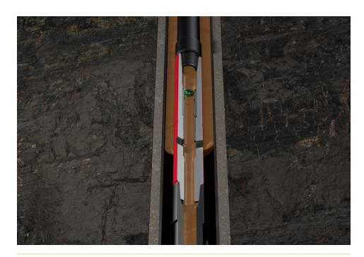
The SuperFill™ II diverter reduces surge pressure to optimize casing run speed.
