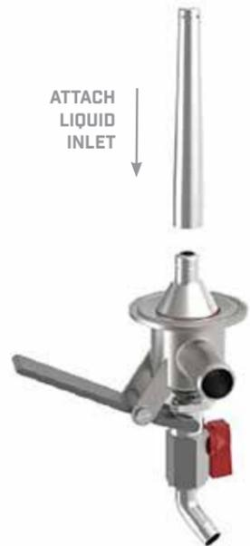
2. Attach the valve to the bottom of the fermenter by inserting the cone plug seal. Then use the tri clamp to tighten it and secure it in place.
