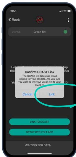
3. You can now view the live gravity and temperature readings from your Tilt device. The GCAST will also start logging the gravity and temperature of your brew every 15 minutes.
