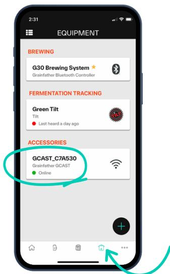
3. Press 'pair' under **G30** configuration. The **GCAST** will now search for a device to link to.
