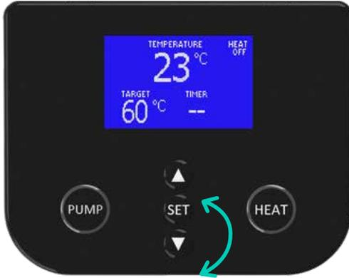
2. Press the up or down arrow to choose an option and press the 'HEAT' button to proceed with your selected option.
