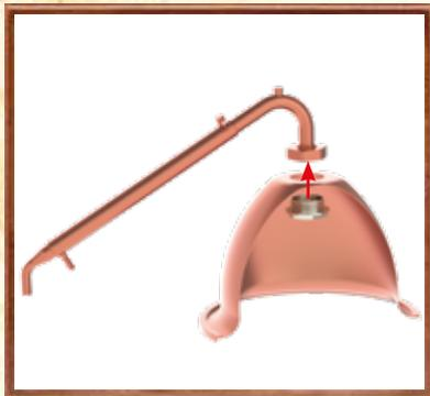
**1** . Attach the copper condenser arm to the copper dome by removing the nut and O ring from the base of the condenser. Sit the condenser on the dome and screw the nut and O ring back into the condenser (check the lid isn't spinning anymore) to firmly attach the dome to the condenser.
