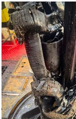
The ESP BHA was located inside 9½-inch casing, above the 7-inch liner hanger at a depth of 10,523 feet. The fishing operation was particularly challenging due to the presence of electrical wire and the unknown condition of the BHA. Jarring was limited to the weakest latching point—the EUE coupling.
