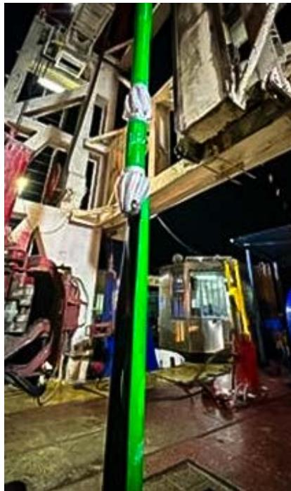
The 7-inch whipstock was successfully set at 5,904 meters with a 66° right-hand side (RHS) orientation. Following completion of the window and rathole, a bottomhole assembly (BHA) with a 5<sup>5/8</sup>-inch OD bit and 5<sup>5/8</sup>-inch OD watermelon mill was run to extend the rathole and ensure sufficient length for the rotary steerable system (RSS) to pass through.
