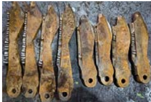
K-Mill tool, and TruEdge inserts after POOH during milling operation.
