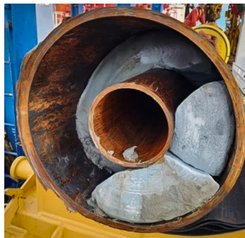
9 \frac{5}{8} inch casing x 24 inch conductor cut
