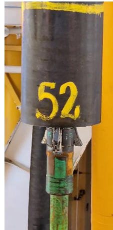
Wellhead and casing conductor retrieved with the ProLATCH System
