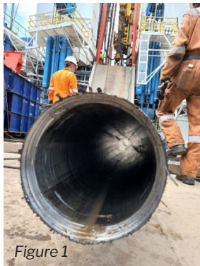
Figure 1: Cut 9 \frac{5}{8} inch Casing 53.5ppf
