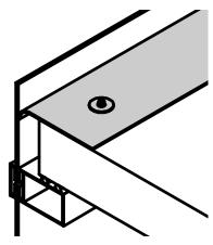
Gasket positioned over sealant and to extend nom. 3 in. beyond edge of slab. Gasket secured in place using nom 1-1/4 in. long by 1/4 in. diameter concrete screws in conjunction with steel fender washers. Fasteners spaced nom. 12 in. OC.
