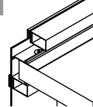
SpecSeal® SIL300 Silicone Sealant applied over backer rod to a min 1/2 in. depth on interior side of wall on top and bottom side of floor.
