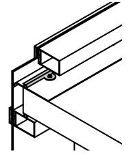
(Optional) Exterior grade silicone sealant applied as required over foam backer rod on top and bottom surface of floor on exterior side. flush with face of concrete floor
