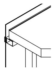
(Optional) Apply nom. 1/4 in. diameter bead of silicone sealant to top surface of floor.
