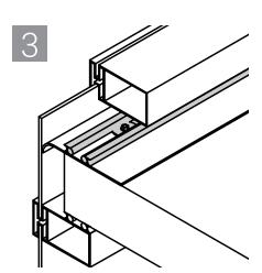
Foam backer rod friction fit into gap between transom and gasket on interior side of wall. (Optional) Foam backer rod friction fit into gap between transom and gasket on exterior side of wall.
