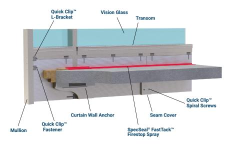
Quick Clip™ L-Brackets: Available for 2" (50.8 mm), 3" (76.2 mm), 4" (101.6 mm), 5" (127 mm), and 6" (152.4 mm) insulation thicknesses
