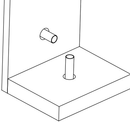
Areas to be protected must be clean and free of oil, loose dirt, rust or scale. Allow product to dry a minimum of 24 hours before exposure to moisture. Consult appropriate manufacturer's drawing for system design requirements. Forming or packing materials are required as an integral part of various system designs.
