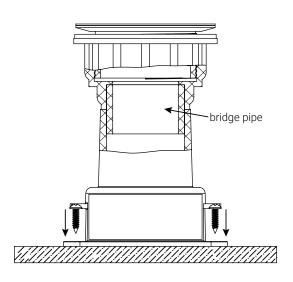
Weld drain body, drain device, and bridge pipe together using appropriate PVC cement. Fasten Drain Device body to plywood forms using steel screws.
