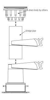
Drain device and bridge pipe to be cut to accommodate for concrete floor thickness. 2" drain body type and style may vary by manufacturer.
