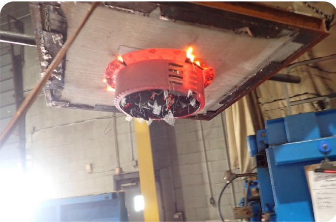
EXC Firestop Collar Following Fire Test and Being Prepared for Hose Stream Test (C-AJ-2995)
