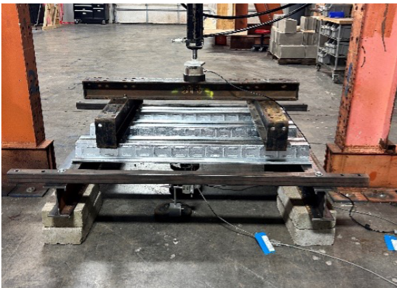
Specimen 1: Standard steel deck panel without concrete, no openings in the deck
