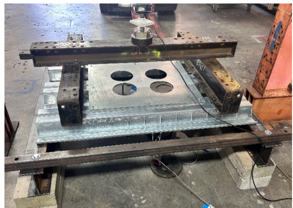
Specimen 4: Steel Deck Panel without concrete, with opening in the deck and a 0.07" standard support plate.
