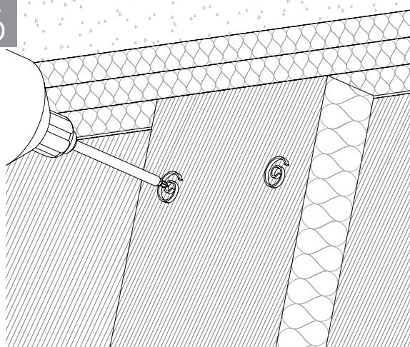
Mullion covers secured to the curtain wall insulation with min 3-3/4" (9.5cm) long galvanized steel spiral screws. Quick Clip™ Spiral Screws installed using a #2 Phillips head drill or equivalent. The number of screws and installation locations as are specified in the applicable UL Systems.
