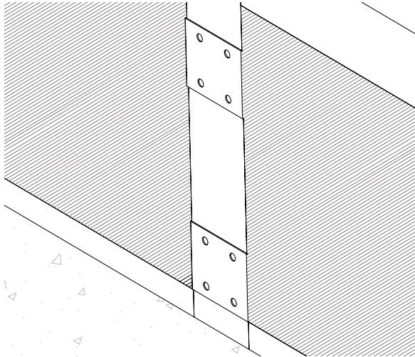
Curtain wall insulation batts to be installed as continuous pieces with one horizontal seam located at the "L-shaped" angle. Curtain wall insulation installed over the Quick Clip™ U- or Z-Brackets flush with the front face of the framing.
