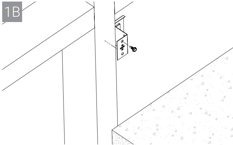
Attach Z-Bracket to mullion (vertical framing) using minimum of one No. 10 by min 1/2" (13 mm) long self-drilling, self-tapping steel screw or as specified in the applicable UL System. Z-Bracket to be located nominally 2" (51 mm) from bottom of sill and 2" (51 mm) from the top of the transoms (horizontal framing) below the floor.
