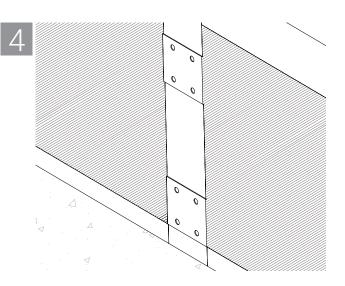
Curtain wall insulation batts to be installed as continuous pieces with one horizontal seam located at the "L-shaped" angle. Curtain wall insulation installed over the Quick Clip™ U- or Z-Brackets flush with the front face of the framing.
