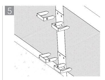
Insert Quick Clip™ Fasteners completely engaging clips at all U- or Z-Brackets on both sides of the framing.
