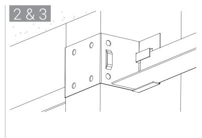
If a L-shaped steel angle stiffener is required by an applicable UL system, the galvanized angle thickness shall be specified. Measure distance between mullions and cut nominal 1-1/2" (38 mm) by 1-1/2" (38 mm) galvanized steel "L-shaped" angles to measured length minus 1/8" (3.2 mm) to max 5/8" (15.9 mm). (Not Shown)
