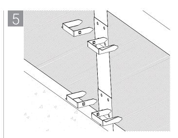
Insert Quick Clip™ Fasteners completely engaging clips at all U- or Z-Brackets on both sides of the framing. Note: Additional steps are required in order to complete the installation. Follow applicable UL System for additional detail on the installation of the Safing System and for the sizing of the Mullion Covers.
