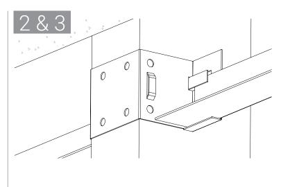
Measure distance between mullions and cut minimum 1-1/2" (38.1 mm) by 1-1/2" (38.1 mm) by min 16 gauge (1.5 m) galvanized steel "L-shaped" angles to measured length minus 1/8" (3.2 mm) to max 5/8" (15.9 mm).
