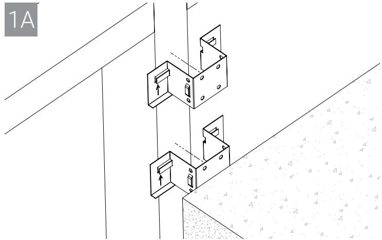
Clip U-Bracket onto mullions (vertical framing) nominally 2" (51 mm) from bottom of sill, flush with the bottom of the floor and 2" (51 mm) from the top of the transoms (horizontal framing) below the floor. U-Brackets lock into place with a strike of a mallet.
