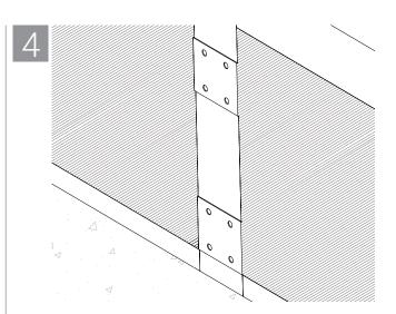
Curtain wall insulation batts to be installed as continuous pieces with one horizontal seam located at the "L-shaped" angle. Curtain wall insulation installed over the Quick Clip™ U- or Z-Brackets flush with the front face of the framing.
