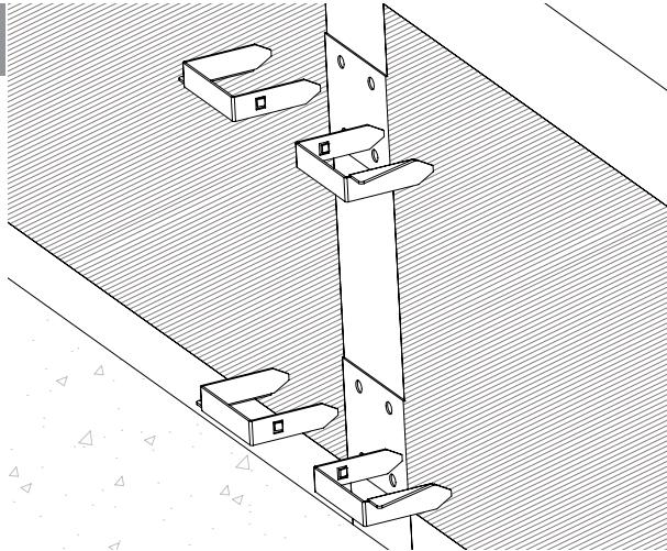
Insert Quick Clip™ Fasteners completely engaging clips at all U- or Z-Brackets on both sides of the framing.
