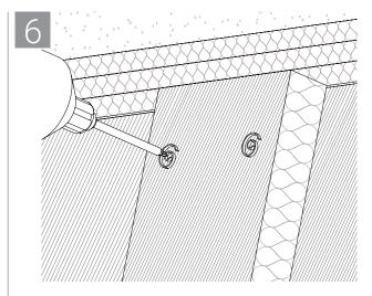
Mullion covers secured to the curtain wall insulation with min 3-3/4" (9.5cm) long galvanized steel spiral screws. Quick Clip™ Spiral Screws installed using a #2 Phillips head drill or equivalent. The number of screws and installation locations as are specified in the applicable UL Systems.
