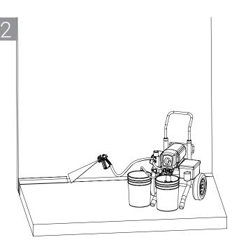
Coating may be applied by airless spray in a single pass as thick as 3/16" (4.8 mm) wet coating depth, although coating thickness requirements vary according to individual design.
