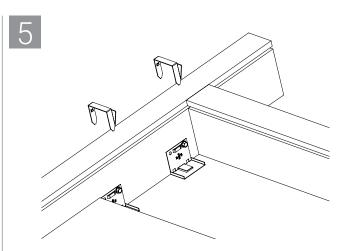
Insert Quick Clip™ Fasteners completely engaging clips at all L-brackets on both sides of the framing. Insulation panel is hidden in the upper part of the image in order to show L-brackets.
