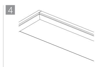
Curtain wall insulation batts to be installed as continuous pieces with one horizontal seam located at the "L-shaped" angle. Curtain wall insulation installed over the Quick Clip™ L-brackets flush with the inner face of the L-bracket.
