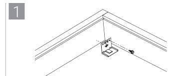
Attach L-bracket to side of mullion (vertical framing) using minimum of one No. 10 by minimum 1/2" (13 mm) long self-drilling, self-tapping steel screw or as specified in the applicable UL System. L-brackets to be located 2" (51 mm) from the bottom surface of sill transoms and 2" (51 mm) from the top surface of the transoms below the floor.
