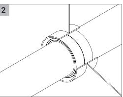
Adjust MWS Marine Wrap Strip positioning such that they are recessed min 12.7 mm from each sleeve end
