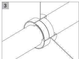
Apply MFS Marine Firestop Sealant over MWS Marine Wrap Strip on both sides of sleeve to a min 12.7 mm thickness, flush with sleeve ends.
