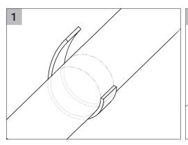
Install two layers of MWS Marine Wrap Strip around the pipe on both sides of sleeve.
