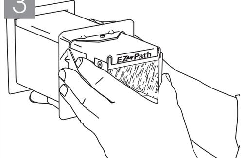
Insert Device into opening and install steel retaining plate and gasket on opposing side of wall. Secure plate to pathway by tightening hex head slotted screws. Ends of device to project equally from wall surfaces.
