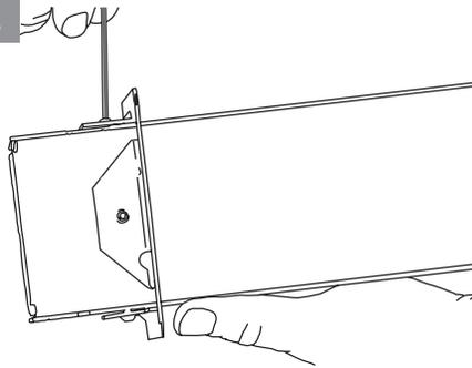
Install steel retaining plate and gasket on one end of device with flanges oriented towards end of device. Secure plate to pathway by tightening hex head slotted screws
