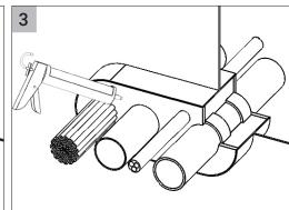
Apply MFS Sealant over MFB Marine Filler Blanket and MWS Marine Wrap Strip (if present) on both sides of sleeve to a min 12.7 mm thickness, flush with sleeve ends.
