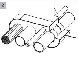
Install MFB Marine Filler Blanket within sleeve to fill all voids around penetrants, recessed 12.7 mm from sleeve ends to accommodate sealant.
